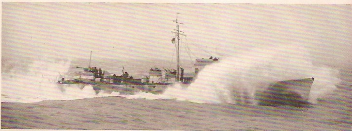
"D" TYPE FAIRMILE of the Royal Navy punching into a head sea in the Straits of Dover. This type is V bottom, faster but not as suitable for bad weather as the "B" type.
